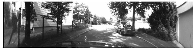
**Figure 8. Cylindrical rectification of the left image in Figure 3. The scene appears similar to the original image but epipolar geometry along lines is obtained.**
