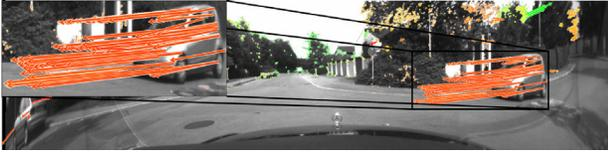
**Figure 14. 6D Vision result for the previous intersection scene two seconds later. The ego-vehicle came to a stop, the vehicle from the right side continues on its path unobstructed by the ego-vehicle.**
