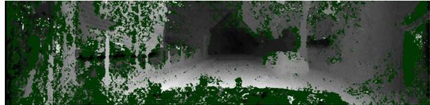
**Figure 10. Global stereo result - unmatched areas are marked in dark green, the closer the object the brighter.**
