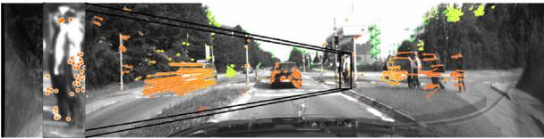
**Figure 15. 6D Vision result for an intersection scene with pedestrians approaching from the right. Since the pedestrians close to the driving corridor came to a stop it is safe to continue driving.**
