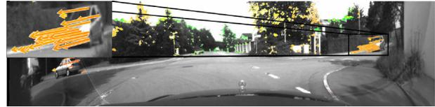
**Figure 13. 6D Vision result for a scene with a vehicle approaching fast from the right side having the right-of-way. The significant lateral motion is detected within 4 frames. Arrow length shows the predicted position in 0.5s. The arrow color encodes distance - red is near and green is far away.**
