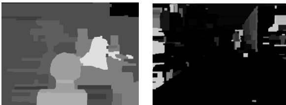
Figure 6: This figure shows the results of BT Stereo on the Tsukuba (left) and Construction-Site Sequence (right). Colour encoding: light = close, dark = far.
